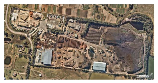
The owner/operators of the site have a preference for the open window method of composting and have applied that method within their business model for over 30 years. Most of materials are collected and prepared for composting at the main facility and then distributed to satellite facilities for maturation and product enrichment and finally, sale. The satellite facilities allow for the increased processing of materials including forest waste, greenwaste, bio-solids and more recently FOGO.
