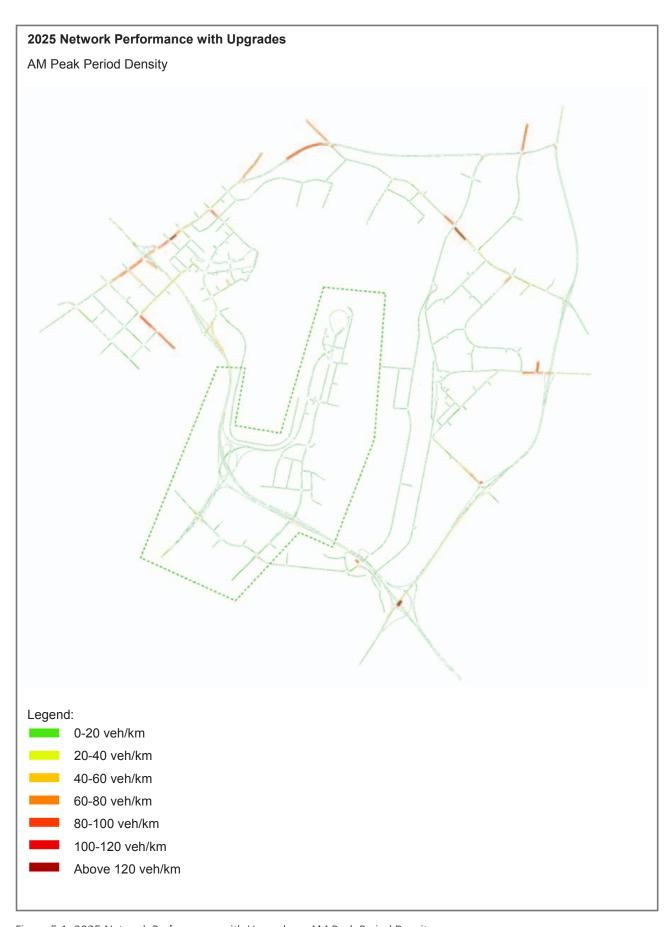
Figure 5.1: 2025 Network Performance with Upgrades – AM Peak Period Density
