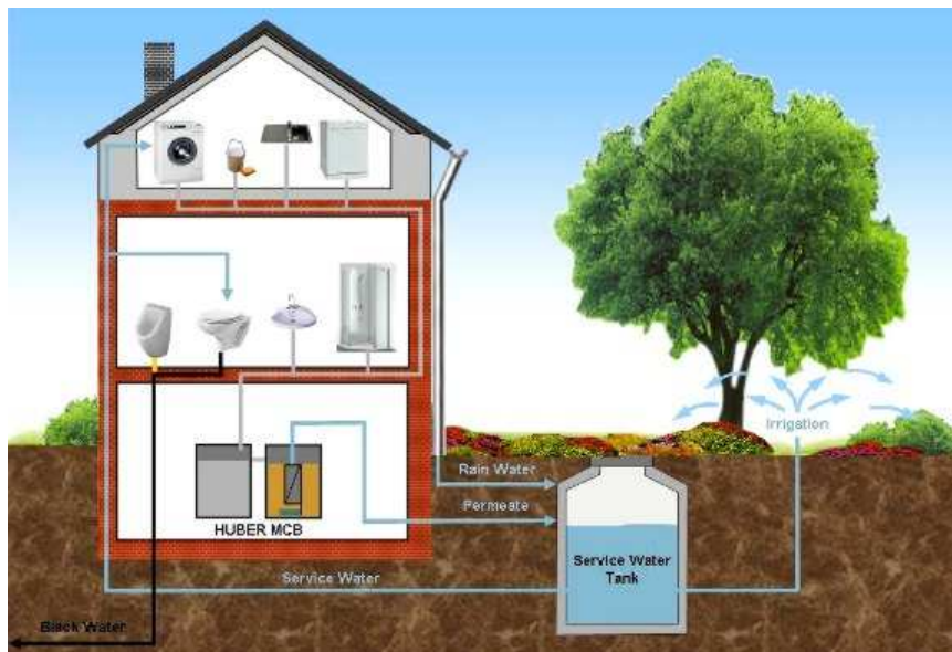
Figure 3 - Simplified schematic of greywater reuse for above ground irrigation (Source: www.ecohomeresource.com ).
