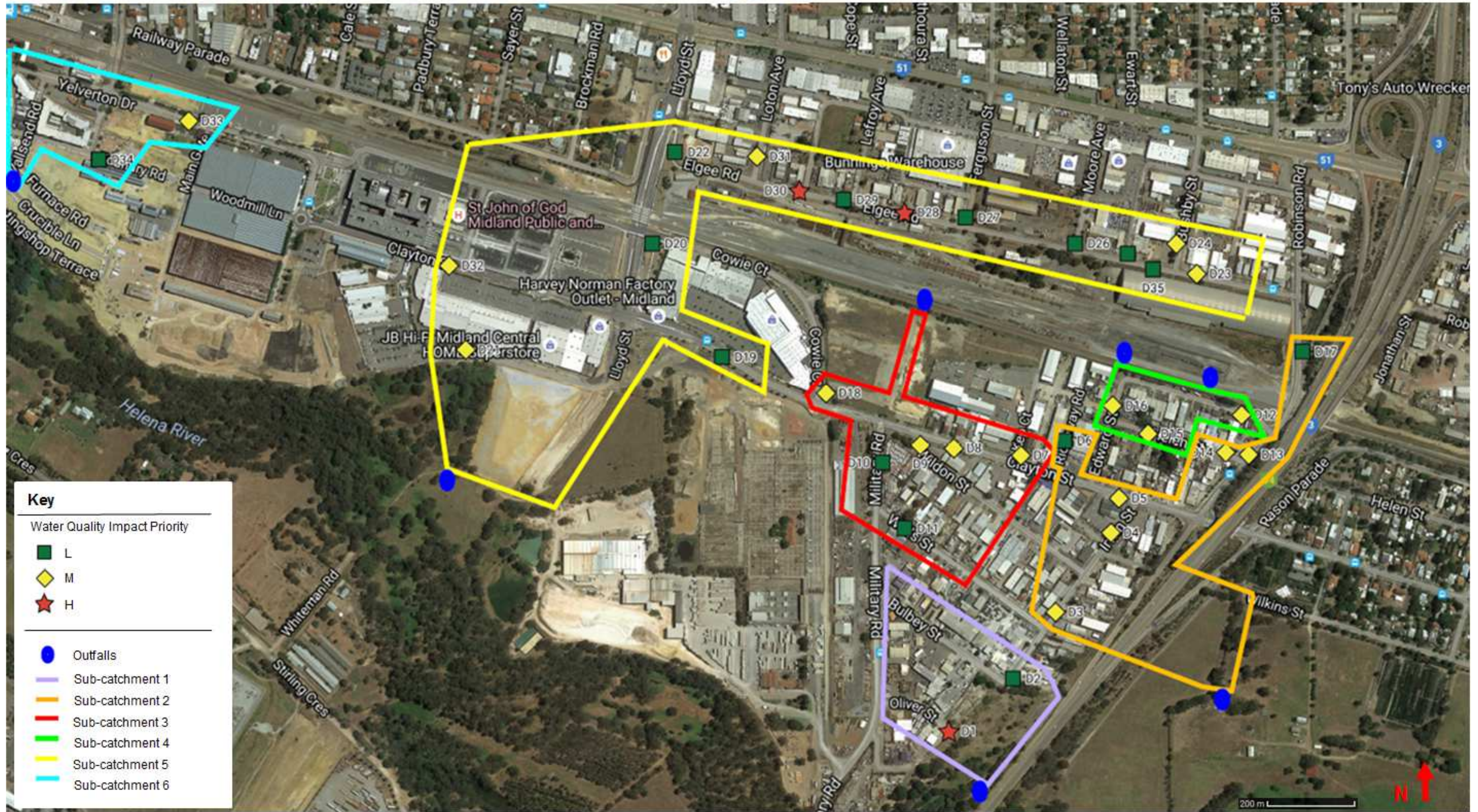
Figure 4: Drain site water quality impact priority and sub-catchments identified within the Bellevue light industrial area
