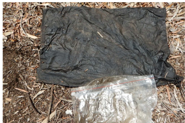
Figure 1: A clean pad (left) compared to a hydrocarbon affected pad (right)
