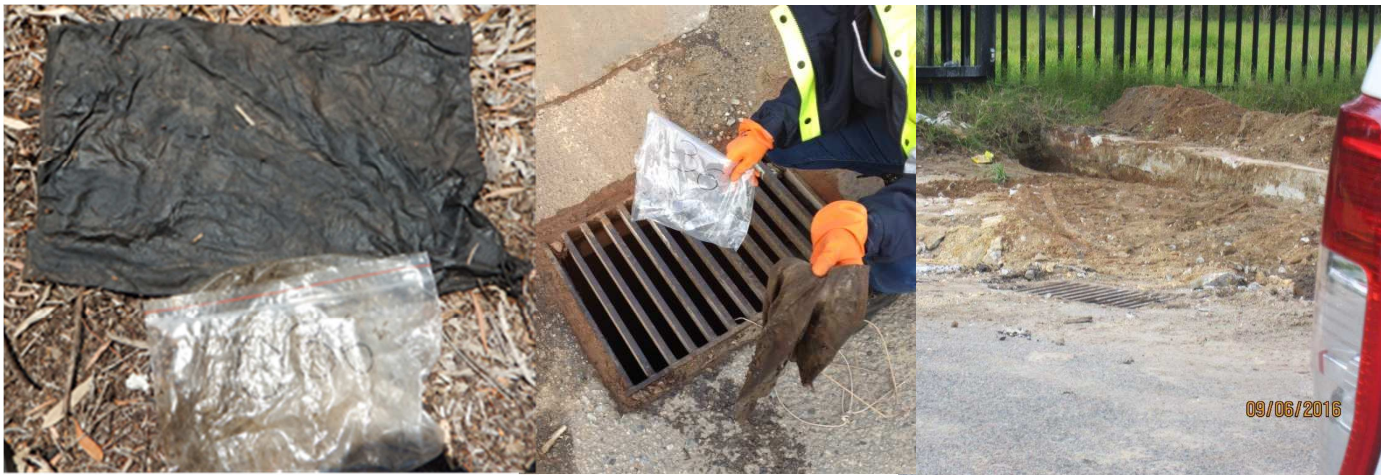
Figure 5: Hydrocarbon pad collected from drain 1 at the end of Oliver Street November 2015, May 2016 and June 2016
