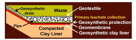
The CLS utilised at the Red Hill Waste Management Facility (RHWMF) is designed and constructed to Industry best practice as detailed above.
