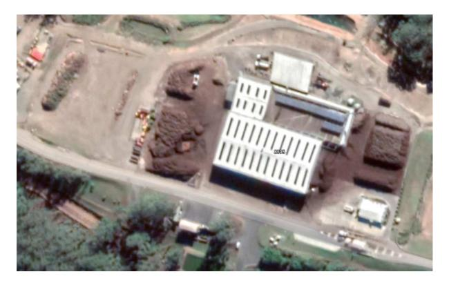
The facility accepts FOGO from Port Macquarie and Hastings plus green waste from separate contractors. In addition to FOGO and greenwaste it also accepts Bio-solids trucked in from Port Macquarie.
