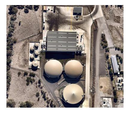
The end product is a liquid and is disposed to the sewer network to seed with bacteria due to its high content. The reduction is of intake material versus out take is 10% for solids and only 2-3% for liquids. This process would not be suitable for FOGO due to its dry content - other AD technologies would be more appropriate. The generator sets have operational and maintenance costs of \$40/hr.
